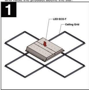
2.) Place one end of the product on the T-bar. Secure the luminaire (fixture) in ceiling using wire or aircraft cable capable of supporting 100lb minimum.
