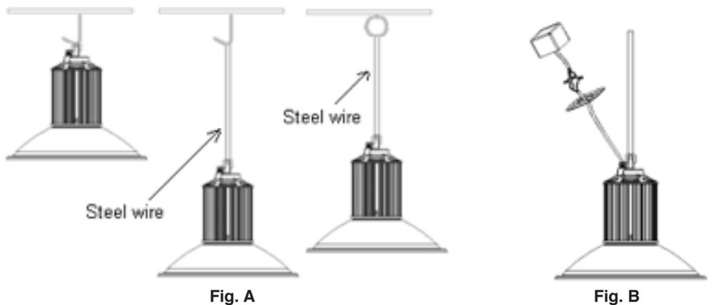
**2:** Make wire connections, connect the power supply that in the outlet box to the black wire to ( L ), White to ( N ), Green to ( Earth) (see Fig. "B")
