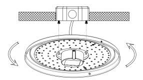
4: Insert wire into junction box, then rotate panel until the screws line up with the screw holes
