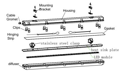
1. Use screwdriver to pry open the clips, without removing
