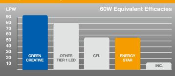
At 94 LPW, this lamp's efficacy is more than 15% higher than the Tier 1 LED A19 60W replacement industry average and exceeds new ENERGY STAR requirements by upwards of 65%. This energy-saving performance makes this lamp a smart retrofit choice for incandescent and CFL bulbs.
