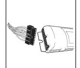
New Quick-Disconnect wiring system.
