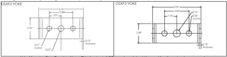
Yoke Mounting Plate Template Note: This drawing is NOT to scale and should be used for dimensional purpose only.
