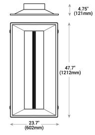
**NOTE:** Use of Expanded Junction Box will expand the depth to  $6.67^\circ$  and Emergency Backup will expand the depth to  $6.30^\circ$ . Use of 347V will increase fixture height by  $1.4^\circ$
