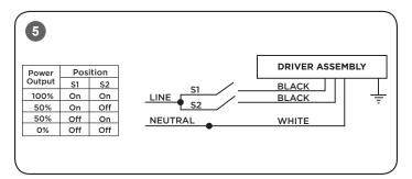
NOTE: (1) DO NOT CONNECT two separate phases of the line voltage to the input of the CR Troffer, the LED driver will be damaged and not covered by warranty.
