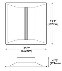
NOTE: Use of Expanded Junction Box will expand the depth to 6.67" and Emergency Backup will expand the depth to 6.30". Use of 347V will increase fixture height by 1.4"
