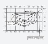
Mounting Height: 25' (7.6m) Initial Delivered Lumens: 2,529 Initial FC at grade
