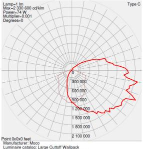
Manufacturer: Moco Luminaire catalog: Large Cuttoff Wallpack Luminaire: Wallpack With Prismatic Glass Lens Lamp catalog: 64 XBDs. LUMINAIRE OUTPUT = 5893 LMS Lamp: Two LED arrays with 32 LEDs each
