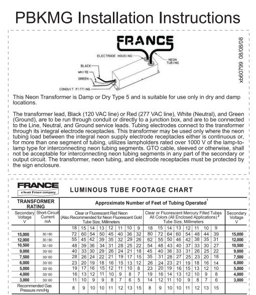
(1) Based on average grade. (2) All enclosed applications. Exposed and extremely cold climates may require footage be reduced by 10-20%. NOTE 1: Deduct approximately 1 foot from above figures for each pair of electrodes.
