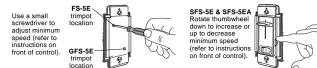
**Note:** If knob has little effect on fan speed, reset minimum speed.
