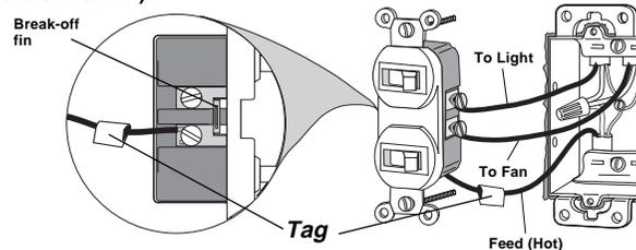
**Step 4** Disconnect switch wires.
