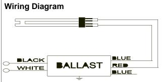
INSULATE UNUSED BLUE LEAD FOR 1000V The wiring diagram that appears above is for the lamp type denoted by the asterisk (\*)
