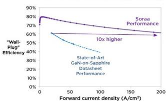
Source: Competitor data sheet, and Soraa internal data at 85°C junction temperature
