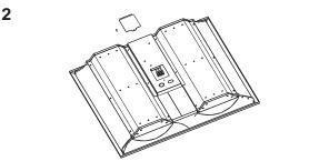
Loosen the screw in the backside channel board with screwdriver, and open one of the knockout holes for threading convenience.
