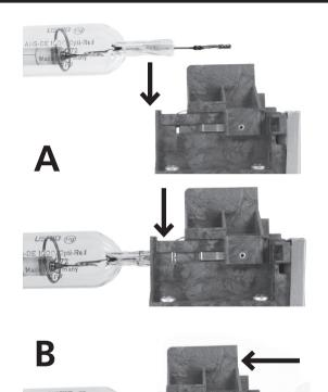
Insert lamp ends into sockets (A).
