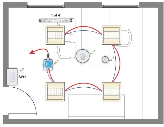
— Line voltage wiring — Low voltage wiring
