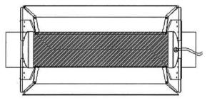
5- You can now turn the reflector right side up and install the 2 v-hooks.
