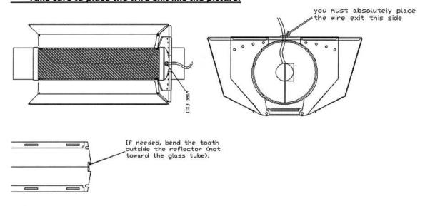
4- Install the second adjustable end cap (A) over the glass tube(E) to cage it inside the assembly.
