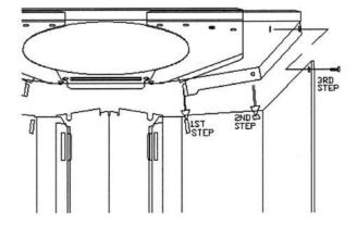
3- Now insert the glass tube trouh the assembled side, until it locks behind the central V reflector(B). The central V reflector(B) is supposed to fit between the glass tube's (E) caps, if it does not fit in, it is probably caused by a small variation in the glass tube's (E) lenth. In this case simply bend the adjustment tooth located at the end of the central V reflector(B).
