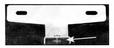
Insert screw into top of bracket and install nut loosely on screw.
