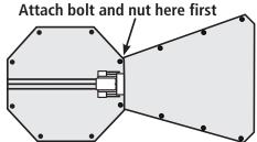
3. Working clockwise, keep attaching a leaf to each side of the octagon. You will need to flex the leafs slightly to get the holes to match up, because the leafs overlap, each bolt will be bolting 2 leafs to the octagon piece.
