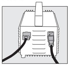
8. Plug ballast into the power supply.
