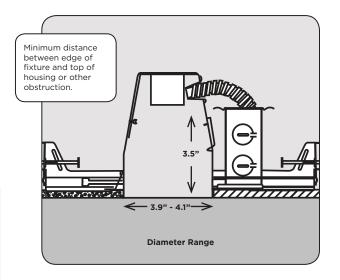
\*Note: Compatible housings should have either an E26 "Edison" base or GU24 base socket, powered by 120V AC and installed according to the National Electric Code and local installation requirements. Always measure existing housings to ensure compatibility.
