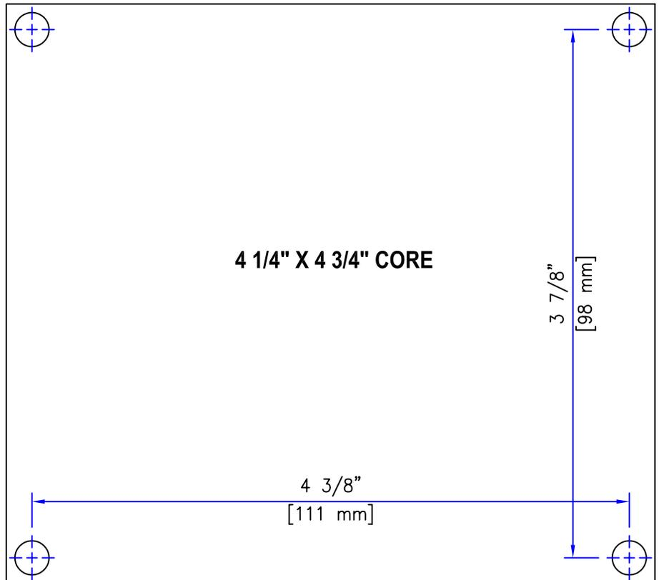
DO NOT REPRODUCE THESE TEMPLATES IN ANY WAY THAT MAY ALTER THE DRAWING SCALE (1" = 1") USED IN THE CORE ALIGNMENT DRAWINGS
