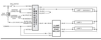
FIG 105 THREE (3) LAMP RAPID START BALLAST
