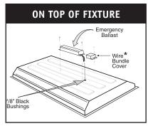
\* For installation on top of the fixture, wire bundle covers (RMC-60) may be required by state or local codes. These covers are available from the manufacturer as an accessory kit and must be ordered separately. Call your local distributor or the factory for complete information.
