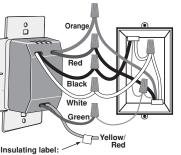
This wire is used in 3-way installations only. For single pole installations do not remove this insulating label.
