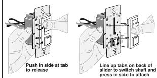
Position the Slide Switch Shaft with the opening in the frame and line up the plastic snaps with the square holes in the strap.
