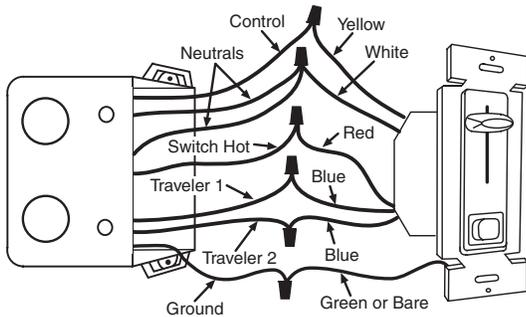
NOTE: If the SF-103P does not turn off, or the unit does not turn on at all, the red and blue wires have been connected incorrectly. The result of the miswire depends on the position of the other 3-Way switch. Check the wiring carefully.
