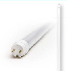
Energetic Lighting's ELT8 series of LED ballast bypass T8 tubes are designed to emulate the look and feel of traditional 4-foot 32 watt fluorescent T8 tubes. Simply bypass the ballast in the existing fixture is all it takes to convert existing fluorescent fixtures into long life LED units. Rated with an L<sub>70</sub> lifetime of at least 50,000 hours, this rugged tube lamp is designed for many years of reliable maintenance-free operation.
