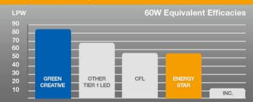
At 84 LPW, this lamp's efficacy is more than 25% higher than the Tier 1 LED A19 60W equivalent industry average and exceeds new ENERGY STAR requirements by upwards of 52%. This energy saving performance makes this lamp a smart retrofit choice for CFL bulbs.
