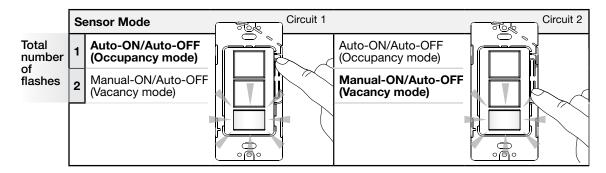
Note: Holding both programming buttons simultaneously will NOT speed up programming. This is the method for programming "Advanced Auto-ON Modes" (see page 8).
