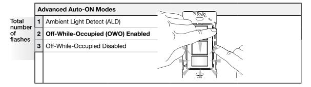
Note: This setting will apply to ALL circuits set to Auto-ON / Auto-OFF (Occupancy) mode, and will not apply to any circuits set to Manual-ON / Auto-OFF (Vacancy) mode. If ALD is selected, the unit will learn from interactions with any circuit set to Auto-ON mode.
