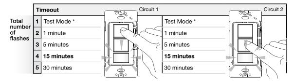
Note on Shortcut: If the desired Timeout for both circuits is identical, both Tap buttons may be held to program the Timeout on both circuits simultaneously.
