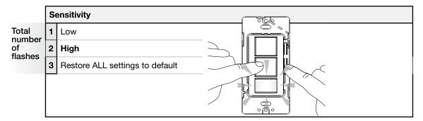
Note: The third flash will reset ALL settings on the unit to factory default. There will be significant delay between the 2nd and 3rd flashes. This is to ensure settings are not accidentally reset while programming sensitivity.
