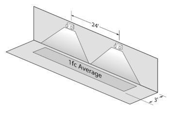
Using multiple units mounted at a typical 7.5' delivers 20' center-to-center spacing on a 6' wide egress path.
