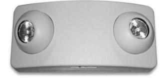
The LL50H Thermoplastic Emergency Lighting Units combine a lowprofile, contemporary appearance with economy and dependability. It's compact, streamlined design features fully adjustable designer 5 watt halogen heads to compliment any environment. Constructed of of an injectection-molded, 5VA flame retardant, high-impact, thermoplastic housing, this durable unit will provide years of reliable service.
