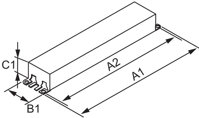
MARK 7 0-10V ELE DIMMING BALLAST (3) F32T8 120-277V
