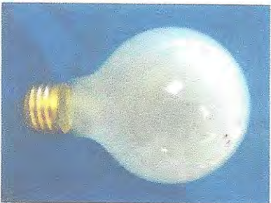
P25/10, 120V/150W E26 Frosted Hard Glass Spot Light Incandescent Lamp 120.7 mm MOL, 76.2mm LCL 200 Hrs, 2850K, C2V Filament
