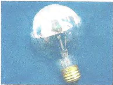
P25/2SB, 120V/150W E26 Clear Silver Bowl Hard Glass Spot Light Incandescent Lamp 120.7 mm MOL, 76.2mm LCL 200 Hrs, 2850K, C2V Filament
