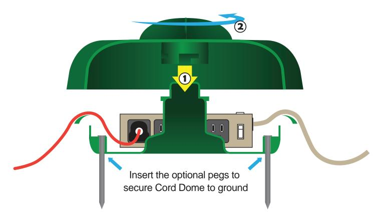
**CAUTION:** Cord Dome provides weather protection and is water resistant, but not water proof. **Do not submerse in water.** Always follow all electrical cord manufacturer instructions.
