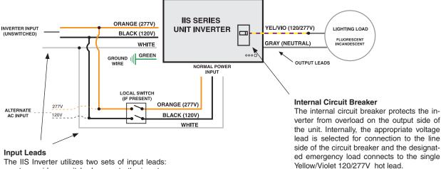
one to provide unswitched power to the inverter system and a second to serve as a normal power input to the lighting load. Any switch for the designated emergency circuit will be present on the Normal Power Input leads. For Emergency Operation Only applications, the Normal Input leads are not needed and would remain disconnected and capped.
