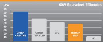
At 86 LPW, this lamp's efficacy is 30% higher than the Tier 1 LED A19 60W replacement industry average and exceeds ENERGY STAR requirements by upwards of 72%. This energy-saving performance makes this lamp a smart retrofit choice for incandescent and CFL bulbs.
