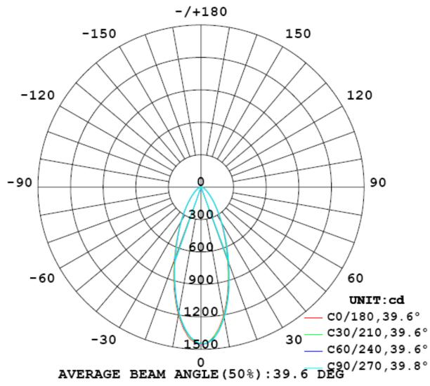
Chart 4: Polar Plot of Normalized Intensity Distribution at Axes of symmetry for 520245
