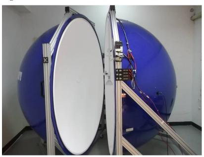
Figure 2: Testing in Integrating Sphere
