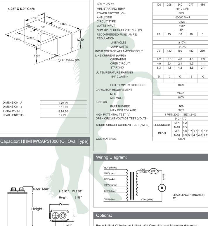
Basic Ballast Kit includes Ballast, Wet Capacitor, and Mounting Hardware only.
