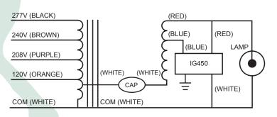
Basic Ballast Kit includes Ballast, Ignitor and Mounting Hardware only. For capacitor option, add Base Model No. and one Capacitor code: **D** = Dry Kit: Ballast + Ignitor + Dry Capacitor + Mounting Hardware W = Wet Kit: Ballast + Ignitor + Wet Capacitor + Mounting Hardware
