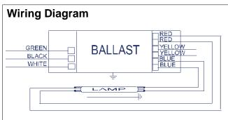
For 1 lamin on eration, do not use vallow leads The wiring diagram that appears above is for the lamp type denoted by the asterisk (\*)
