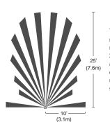
The WN-100 has a coverage range of 180 degrees and a maximum coverage area of 300 ft<sup>2</sup>. To maintain its coverage capacity and optimally detect motion, the WN-100 must have a clear and unobstructed view of occupants.
