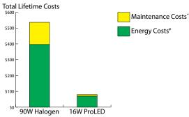
\*Maintenance costs based on 15 minutes to replace the lamp at \$40 per hr over the life of the ProLED lamp.
