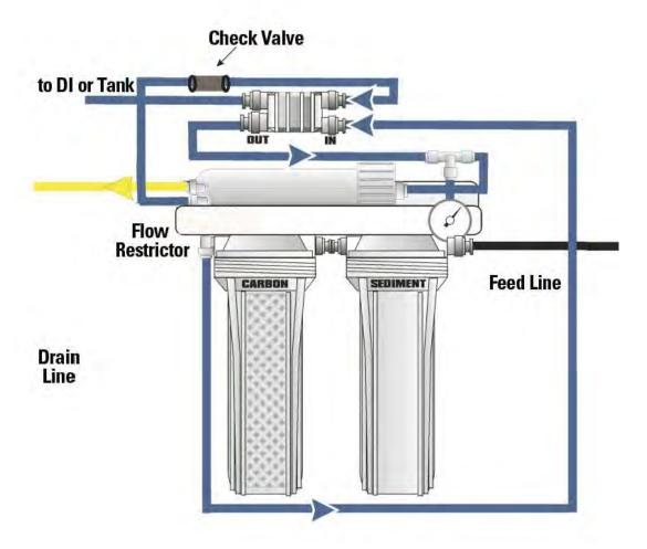
Installing the ASO valve as seen in the Diagram will allow you to make water automatically with the help of a float valve or other external shutoff device.
