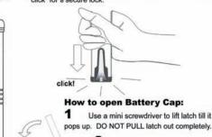
2 Use the thumb to push Cap forward as shown. Turn over to the front and pull Cap out completely.
