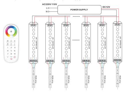
2. Per controller are powered by one power supply independently:
