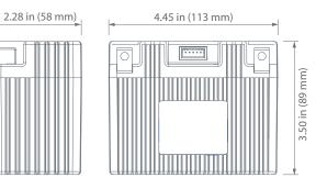
**L:** 4.45 in (113 mm) W: 2.28 in (58 mm) **H:** 3.5 in (89 mm) Tolerances are +/-0.04 in. (+/-1mm)
