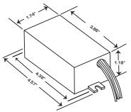
Center line to center line is .16" less than end to end on models with mounting feet.
