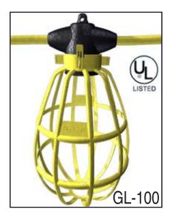
GL100-142 is the latest in our extensive line of Temporary Lighting solutions. Indoor / Outdoor hard Usage 14/2 SJTW (300V) round cord with yellow pvc jacket. 100ft total length with 10 molded lampholders, one every 10ft on center. Each unit includes10 heavy duty yellow plastic lamp guards (Bird Cages) which are uniquely designed for superior performance and extended life. U.L. Listed, N.E.C., OSHA Available in 14/2, 14/3, 12/2 & 12/3 constructions.
