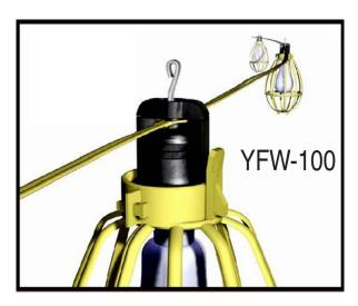
YFW-100 is a basic flat wire unit manufactured with 14AWG stranded flat wire AWM style (600V), and a "pin" type lamp holder every 10ft on center. Each unit includes 10 heavy duty yellow plastic lamp guards (Bird Cages) which are uniquely designed for superior performance and extended life. N.E.C., OSHA approved.
