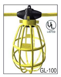
GL100-142 is the latest in our extensive line of Temporary Lighting solutions. Indoor / Outdoor hard Usage 14/2 SJTW (300V) round cord with yellow pvc jacket. 100ft total length with 10 molded lampholders, one every 10ft on center. Each unit includes10 heavy duty yellow plastic lamp guards (Bird Cages) which are uniquely designed for superior performance and extended life. U.L. Listed, N.E.C., OSHA Available in 14/2, 14/3, 12/2 & 12/3 constructions.
